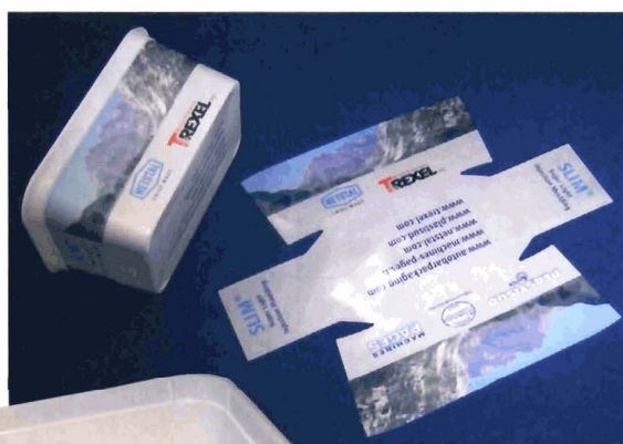
Seen at K 2007 - an in-mould labelled Autobar Packaging SLIM "Super Light Moulding" in the form of a 500g PP container moulded on an Evos machine on the Netstal stand. The process used Trexel's MucCell microcellular physical foam process with cycle time 5 secs in a 4*4 Plasticsud cavity mould with handling equipment from Pagès
